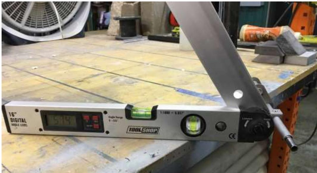
57 degrees  $\pm$  2 degrees is correct angle. Steel handle is hidden, behind digital angle, lying flat on table.
