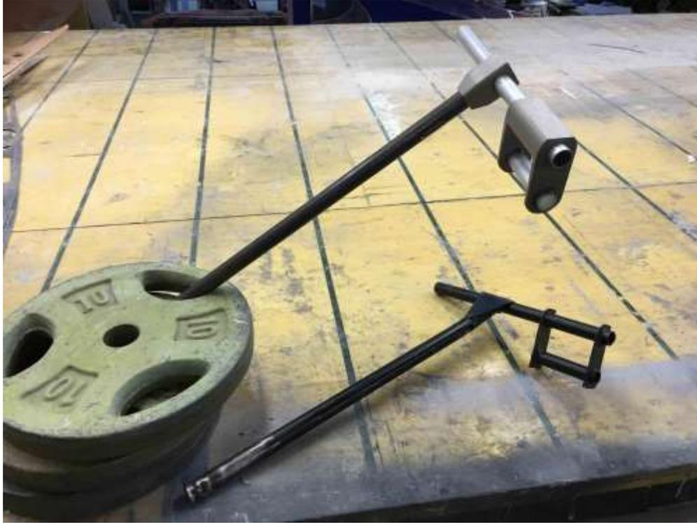
We used weighted base to allow angle to hold during epoxy cure. Predecessor welded part (obsolete) also shown.
