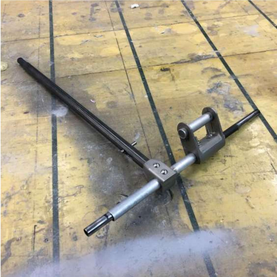
8. Insert spring and nylon pushrod into 9/16" handle steel tube with slots. You may need to trim end of main steel tube to allow full range of "push button" motion. Roughen steel pin and insert through hole, using small amount of 2216 epoxy to lock position.
